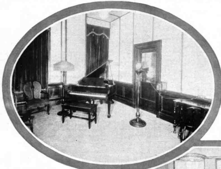
Above—Where the music you hear nightly from WBAP is produced. The studio is soundproof and acoustically perfect, having been corrected by leading engineers. A two-inch layer of felt on walls and ceiling deadens all echo
